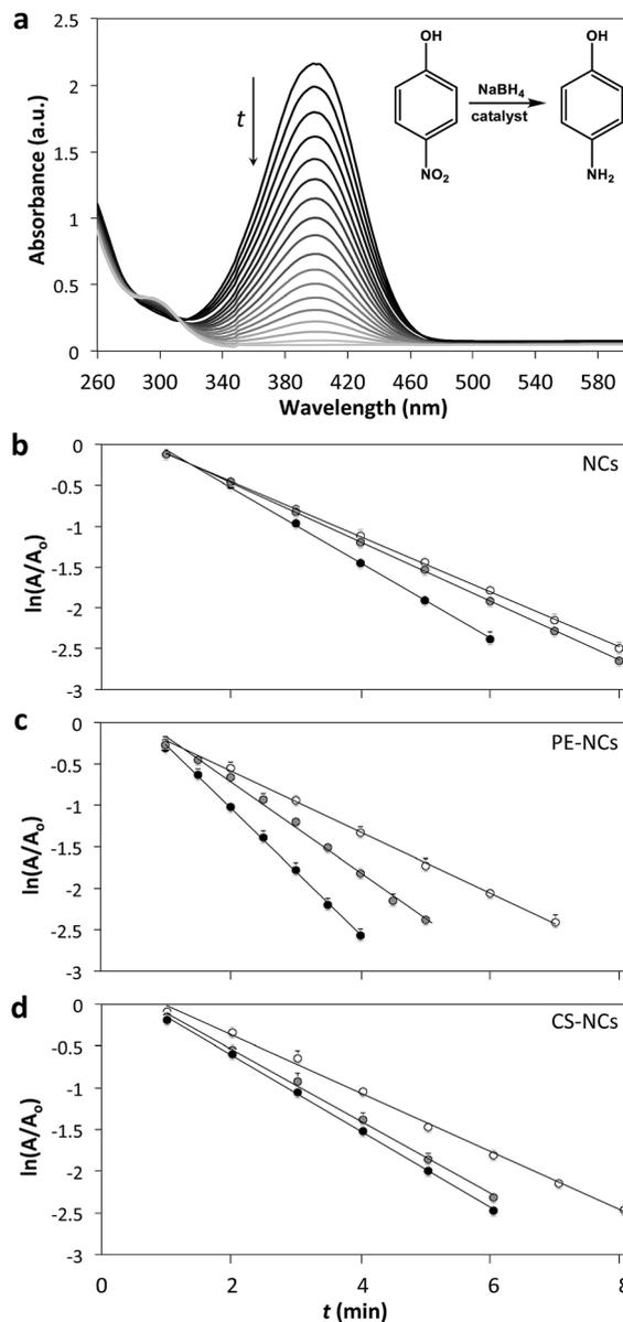
Fig. 2 (a) Evolution of the absorption spectra in the course of 4NP reduction. Inset: reaction of the reduction of 4NP. (b–d) The dependence  $\ln(A/A_0)$  vs.  $t$  for 4NP reduction in dark (open symbols), under illumination at 450 nm (black symbols) and 532 nm (grey symbols) using NCs (b), PE-NCs (c), and CS-NCs (d).
